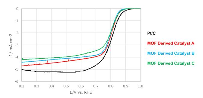
Electrochemical properties of MOF derived catalyst compared with commercially available Pt loaded carbon catalyst measured with rotation disk electrode.
